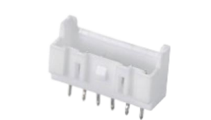
JL2515S系列 2.5mm间距 双锁车规级WTB单排180°针座 Spec: JL2515S Series 2.5mm Double Lock Gauge WTB Single Row Straight Installation type:Through-hole
